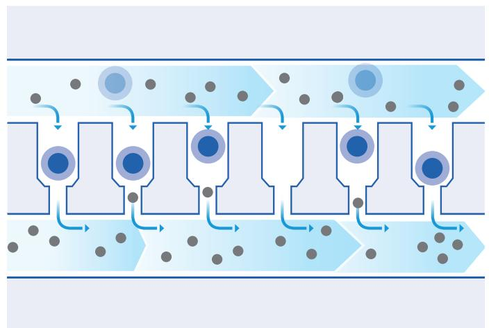
**Figure 3:** Size-based enrichment of CTCs. A schematic of the microfluidic chambers used to capture CTCs based on their size.
