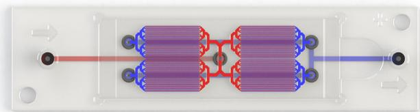
**Figure 5.** A schematic representation of the Celselect Slide. Blood sample (red, left) flows through the microchambers in the Celselect Slide and exits to the waste port (blue, right)
