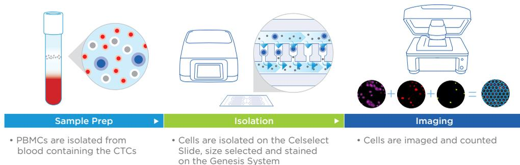
**Figure 4.** Cell Enumeration Workflow. Blood is directly added to the sample inlet; CTCs are isolated in the Celselect Slide while the smaller RBCs and WBCs pass through to the waste. CTCs are processed and immunostained directly in the slide. Subsequently, CTCs can be visualized and counted on the slides using an automated fluorescent imager. Contamination from larger WBCs can be excluded through image analysis.
